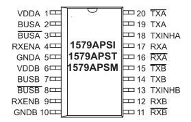
20 Pin Plastic ESOIC - WB package
